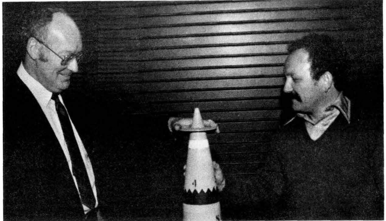
EXAMINING A TEST SHELL are Ben Benedetti (8241), left, and Danny Mitchell (8163). The pair recently solved the riddle of why a spinning shell descending on a parachute tends to nutate (turn upside down). This unit is atypical in that it has a spoiler disk attached to the nose to increase aerodynamic drag and slow the projectile so that it reaches only 30,000 feet instead of the maximum altitude of 70,000 feet.
